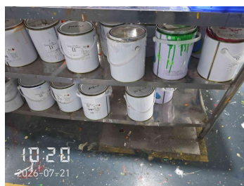
Chemical without secondary container.jpg
